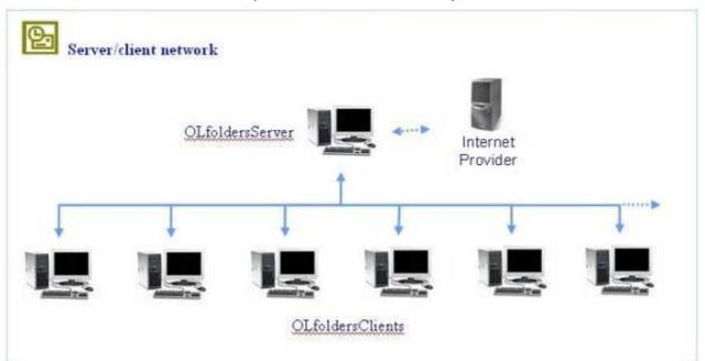
In a client/server structure, only one server is installed. For OL folders it does not make a difference if the server computer is a dedicated server or any workstation.
